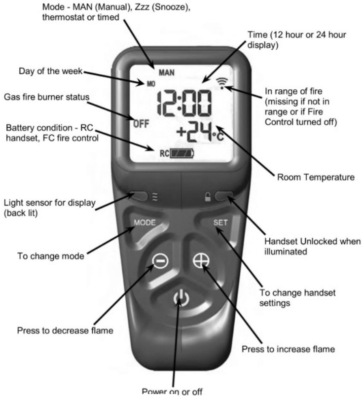
Fig.3 Remote control handset
